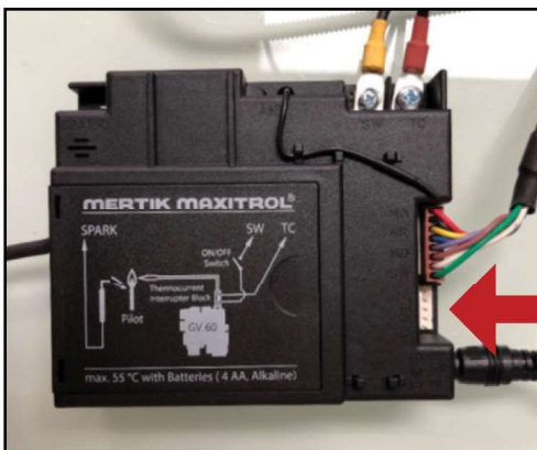
Image 1: Location of wall switch harness connection indicated by arrow
