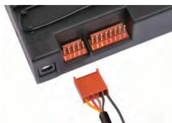
Image 3: Insert plug connector into the receiver.
